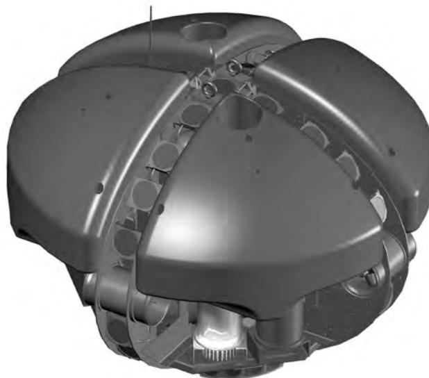
Final DEPTHX design in assembled form. Because of the foam top covers, the center of buoyancy is higher than the center of gravity, so the vehicle is stable in two of its three possible motions.
