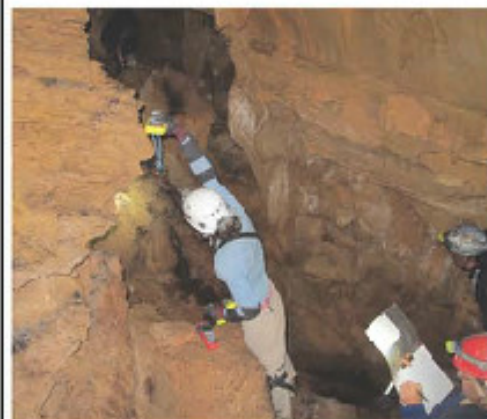
Coel on point surveying with the DUSI and Marion sketching the cave map
