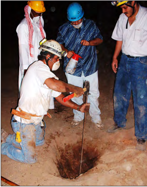
Figure 5. Measuring the depth of the loess bed at the second sampling point.
